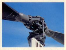
Schweizer uses a three-blade system (below), while Robinson uses two blades. The Robinson rotor is greatly simplified and uses Nylon and Teflon bearings, eliminating all grease fittings. Thus, maintenance costs are expected to be lower.
